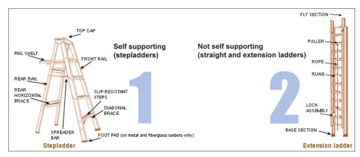
Prior to using the portable ladder, inspect it to be sure that it is in good working order. During this inspection, make sure the ladder meets the following four criteria. If the ladder fails to meet any of these criteria, do not use it:
