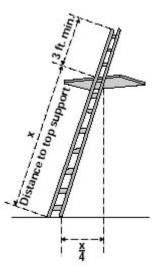
When climbing the ladder, you must maintain three points of contact with the ladder (a hand and two feet or two hands and one foot) at all times. You must have your hands free when climbing. Any equipment you are carrying to the roof must be attached to a belt or carried in a bag/backpack.
